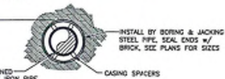
SECTION BORING DETAIL
